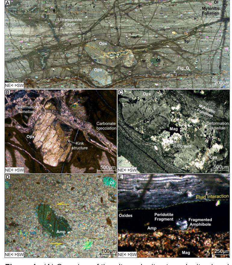
Opx porphyroclast with kink structure and Cpx exsolution ) Opxporphyroclasts bypassed by mylonite folia served the formation of subgrains associated to Mag and Op minerals; (D) Amp bypassed by the mylonitic foliation (G) Fluid Reaction Band.
