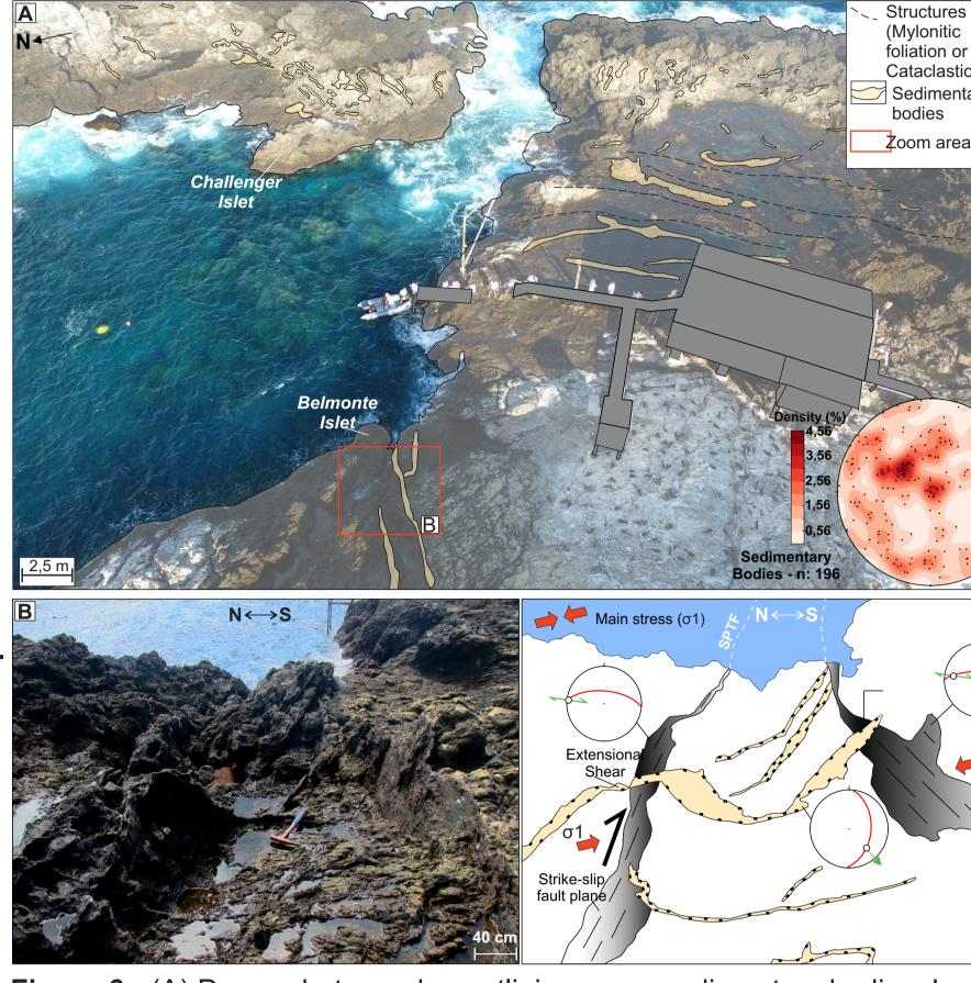
Figure 6 - (A) Drone photographs, outlining some sedimentary bodies. Lower hemisphere, equal area projection indicating the direction of sedimentary bodies Zoom area of the strike-slip fault zone with a obligue component, alongside sional shears oblique to the main fault zone.
