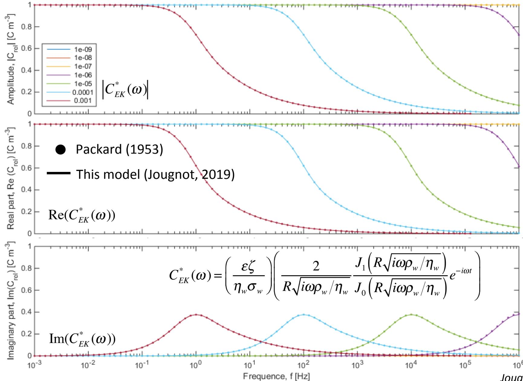
Packard (1953) proposes an analytical solution for a given capillary
