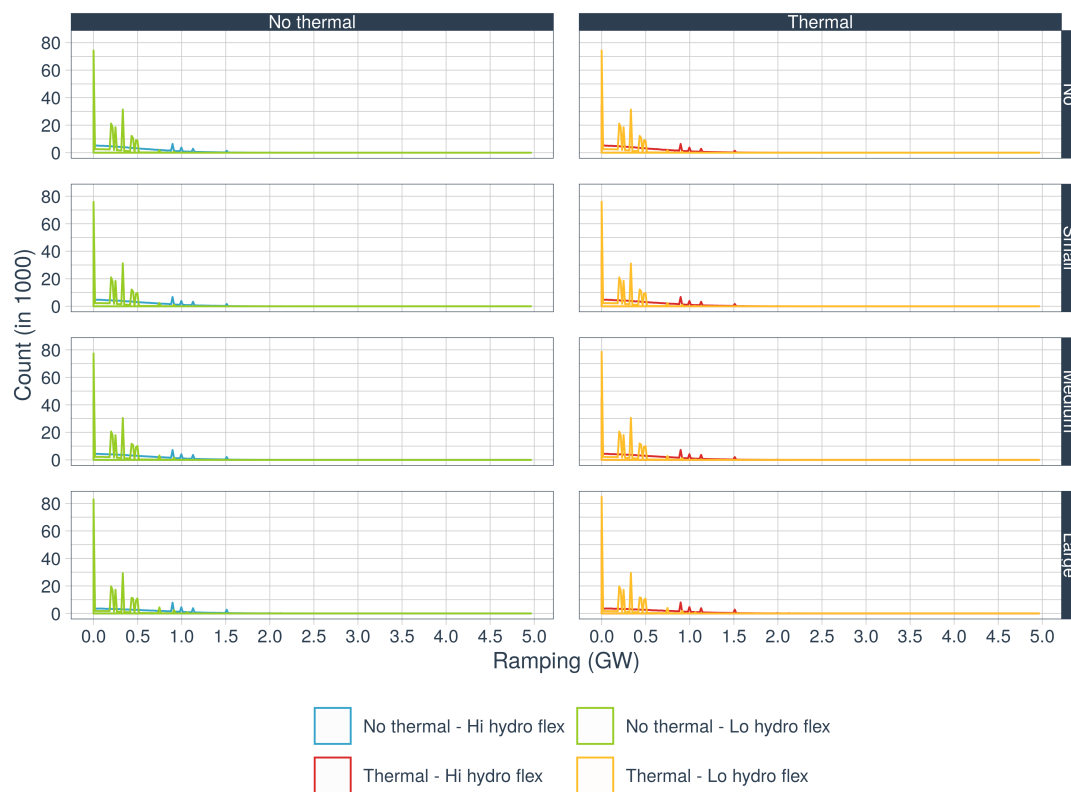
Figure A.12: Density plots of hourly hydro ramps over for all scenarios. Panels left NO THERMAL and right THERMAL, from top to bottom: electrolyzer capacity.
