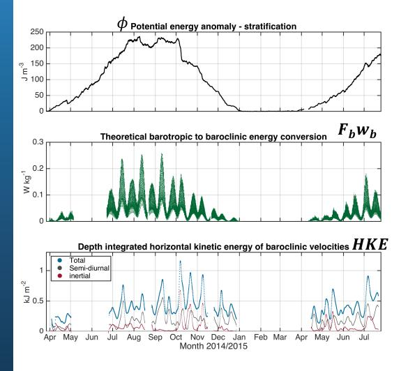
$F_b w_b$  intuitively follows the seasonal cycle of N<sup>2</sup> (or  $\Phi$  here) and is modulated by the spring neap variability of the barotropic velocity.
