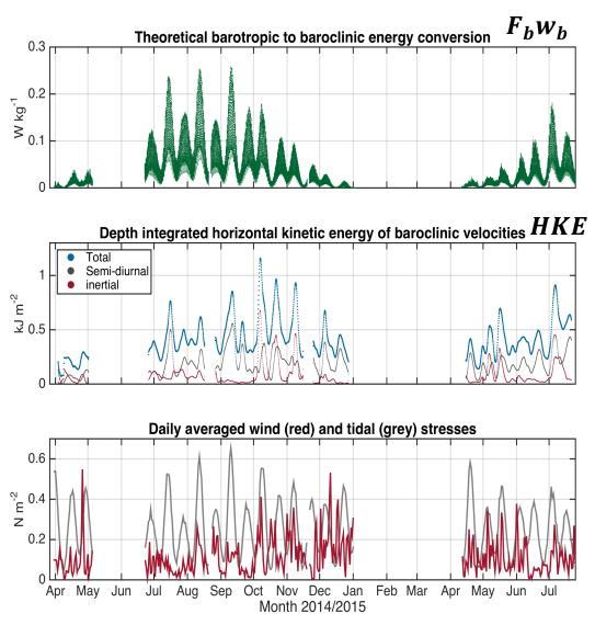
While energy contribution from the semi-diurnal internal tide ( $HKE_{semi-diurnal}$ ) follows the overall pattern predicted by  $F_bw_b$ , we find that inertial oscillations ( $HKE_{interial}$ ) potentially supplied the extra energy evident in autumn 2014 which is in good agreement with increased wind speeds compared to spring and summer periods.
