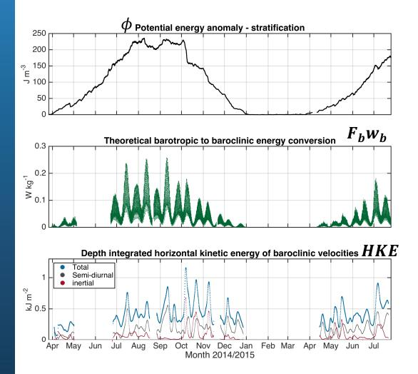
The observed seasonality in the internal wave energy is generally consistent with the theory of internal tide generation. Following Nash et al. (2006) the total rate of work of the barotropic tide interacting with topography is given by the product of the Baines (1982) body force ( $F_b$ ) and the barotropically induced vertical velocity ( $w_b$ ), which Nash et al. (2006) combines as:
