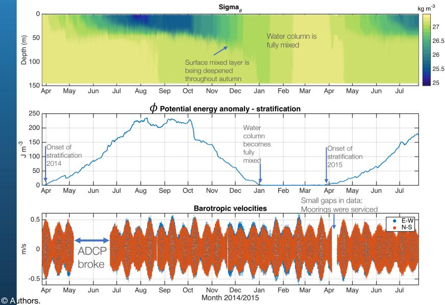
The overall pattern in density structure observed at CCS showed a typical seasonal cycle of stratification.
