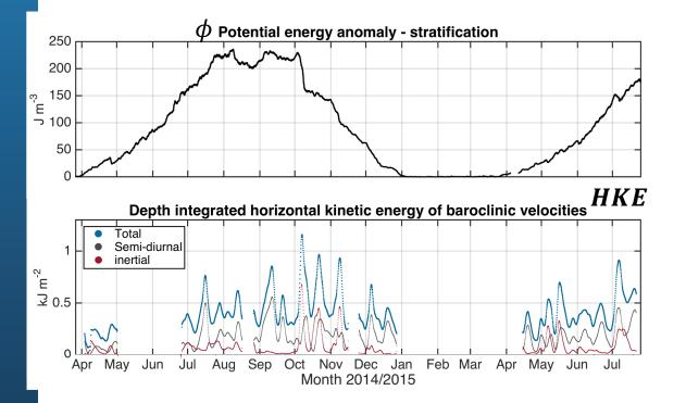
To analyse the seasonality of the internal wave field effectively the total depth integrated kinetic energy of the horizontal baroclinic velocities was calculated: HKE<sub>Total</sub>.
