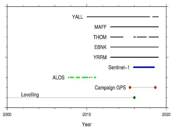
Figure: Black lines are GNSS stations, blue and green are SAR, red are repeat GPS observations, dark green is repeat levelling.
