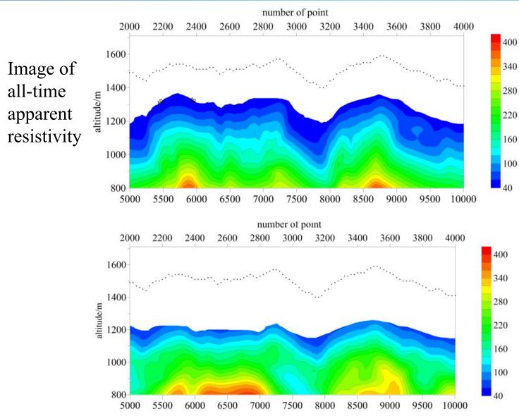
The quasi-resistivity calculated by BP neural networks slightly larger than the results from the all-time apparent resistivity algorithm, which is consistent with the imaging results of the theoretical model. Similarly, the quasi-resistivity isocline from the BP neural network has several mutation bands, which are also caused by the uniform half-space model of the training sample set.
