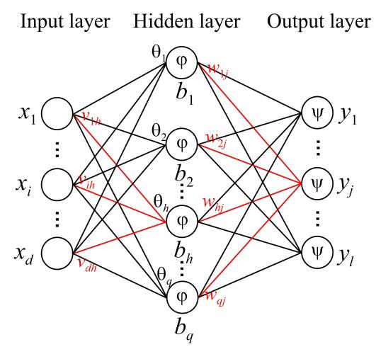
Three-layer BP neural network structure diagram
