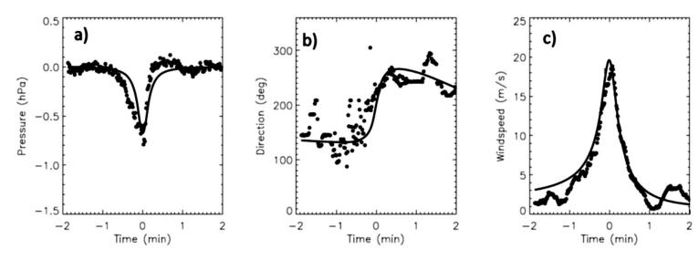
• An example of pressure (a), wind direction (b) and speed (c) measurements for a dust devil encounter in New Mexico during a month-long single-station survey in 2014. Data points are acquired at 1 s intervals, and the curves are a simultaneous fit to the three parameters by an analytical vortex model (from Lorenz, 2016).
