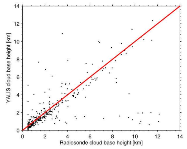
$\Rightarrow$  An overall agreement between the cloud base height is reached from both instruments with a correlation coefficients of 0.73.
