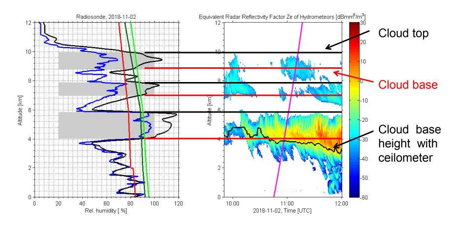
⇒ The three-layer clouds determined with radiosonde in term of relative humidity with respect to ice are in good agreement with the miraMACS results
