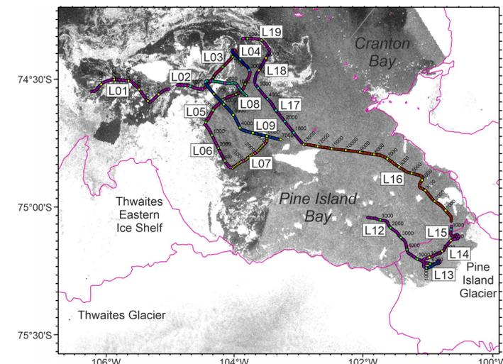
Fig. 6. Locations of high-resolution seismic reflection profiles collected on cruise NBP20-02 overlaid on Sentinel-1 SAR image acquired on March 9th, 2020. Common mid points are annotated at intervals of 1000. Magenta lines are 2016 coastline and ice shelf fronts from the Antarctic Digital Database of the Scientific Committee on Antarctic Research.
