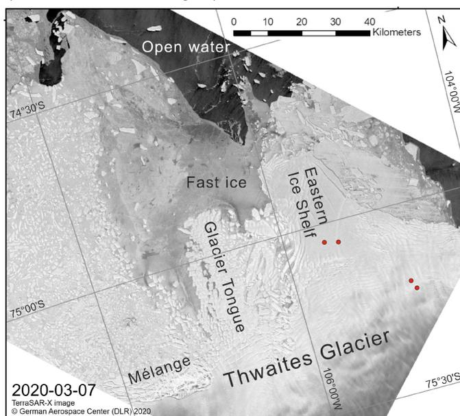
Fig. 2. TerraSAR-X image of Thwaites Glacier area on March 7th, 2020, provided by the German Aerospace Center (DLR). Red dots mark locations of sediment cores recovered from beneath the ice shelf via hot-water drilled holes.
