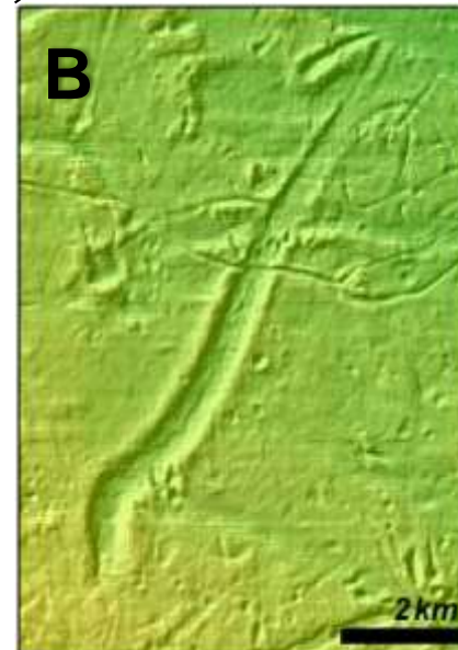
Fig 7. A) Shade-relief map of the seabed (depth converted to meters) showing numerous iceberg ploughmarks. B) Detailed of the shade-relief map of the seabed showing crosscutting relationship between two iceberg ploughmarks found in the study area.
