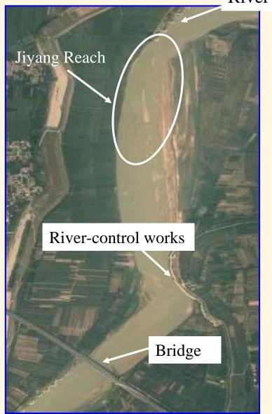
Based on the characteristics of the wandering river reach, a change of the upstream flow direction will make the mainstream directly scour the left bank due to the upstream rivercontrol works and bridge piers. Therefore, for a long time, the riverbank has been attacked by the mainstream and scoured by the backflow due to the downstream control works.
