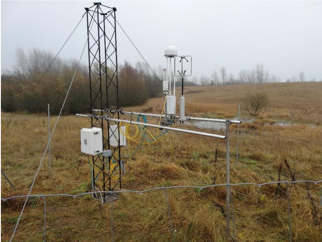
Figure 2. Setup of the eddy covariance instrumentation at Skellingsted landfill. Instruments shown include an open-path CH 4 analyzer, a 3-D sonic anemometer, and an open-path CO 2 /H 2 O analyzer.
