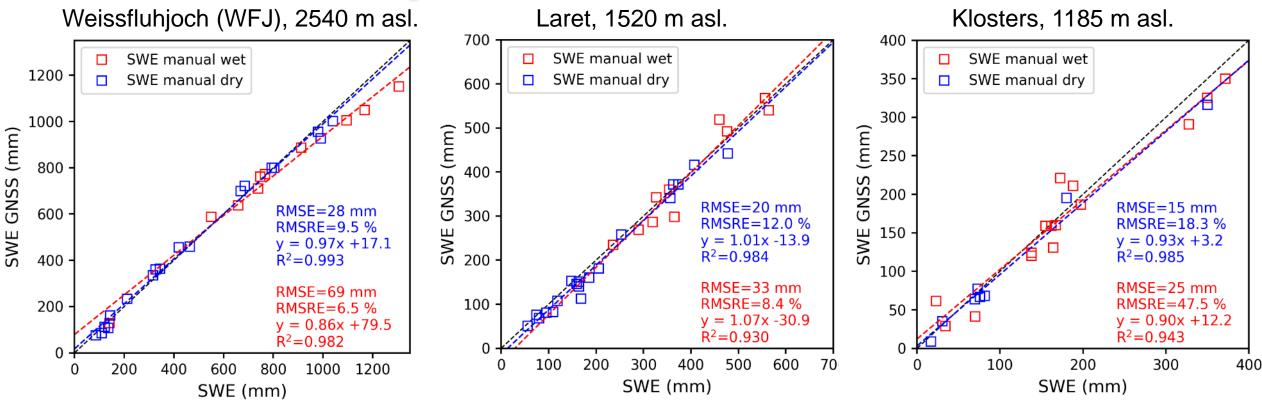
• GNSS-derived values of SWE agree well with manual observations of SWE for both, dry and wet conditions.
