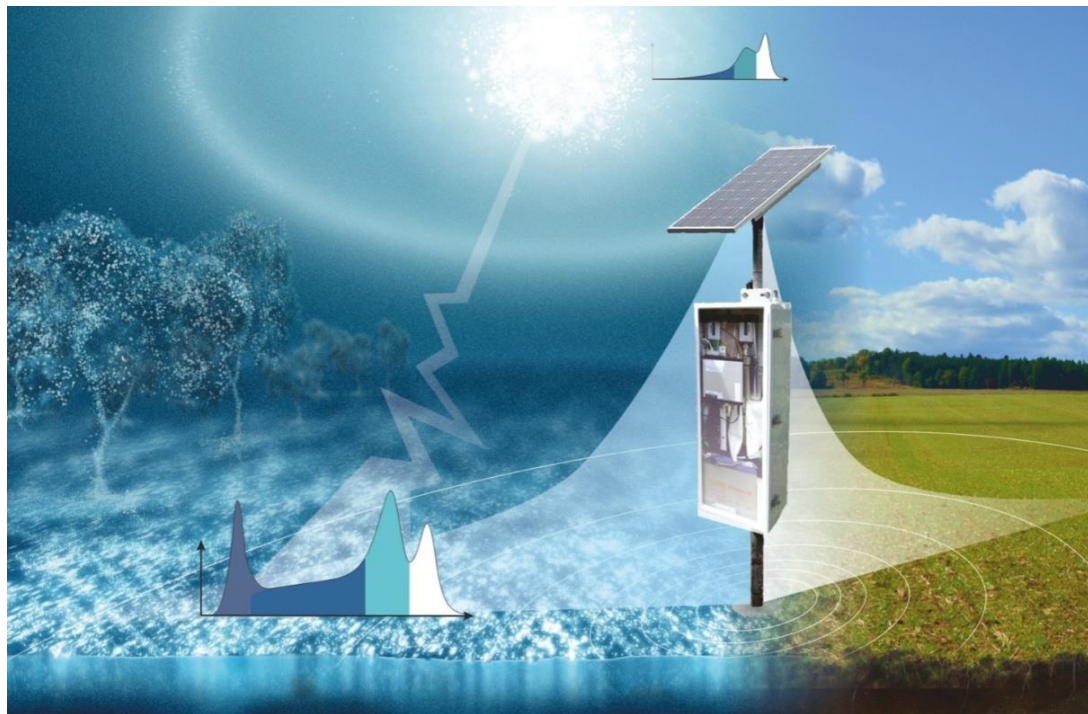
CRNS probe installed at a height of 1-2 m with its exponentially decreasing footprint. Cosmic-Ray Neutrons are generated in air and soil which leads to the prominent CR spectrum with its 3 peaks.
