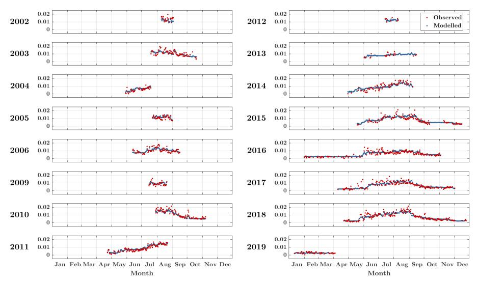
Time series of daily means of CH<sub>4</sub> fluxes F<sub>CH4</sub>. Gap-filled by regression tree model. (Rößger et al., in prep.)
