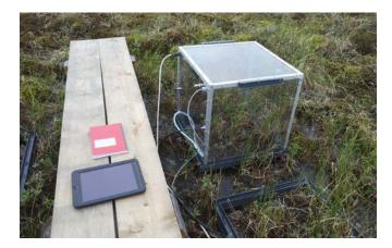
Small-scale CH<sub>4</sub> flux measurements by transparent closed chambers and an Ultraportable Greenhouse Gas Analyzer (UGGA 30-p, Los Gatos Research)
