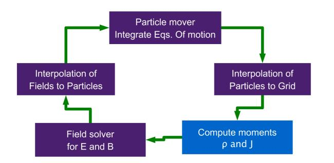
Solution 1: Explicit PIC  $c\Delta t < \Delta x$  $\omega_{pe}\Delta t < \Delta x$  $\Delta x < \zeta \lambda_D$
