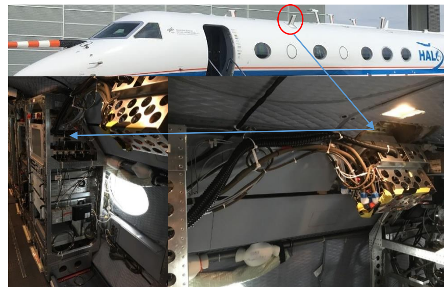
Figure 1: Photo on the top is the view from outside HALO aircraft where the highlighted place is the inlet for the instrument; the photo at the show the PerCEAS instrument and the part of inlet inside the aircraft cabin. The arrows indicate the sample flow direction.
