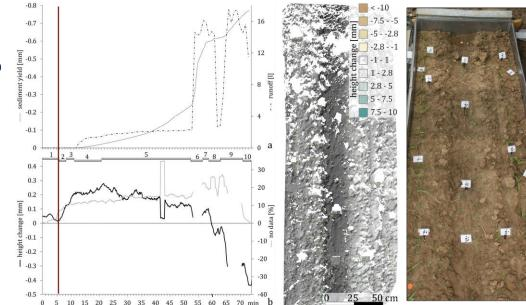
With SfM measured changes during rainfall simulation compared to measurement at system outlet
