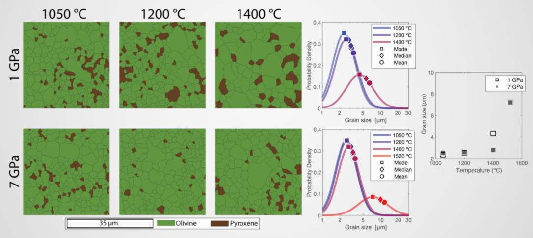
Grain growth is slow at low temperatures (≤ 1200 °C). At 1400 °C, grain growth rate is substantially higher at 1 GPa than at 7GPa.
