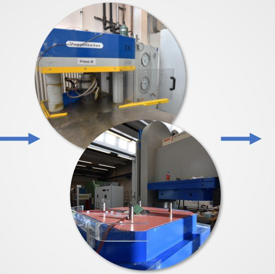
Grain growth experiments were performed using **Piston Cylinder** (19 mm assembly) and **Multi-Anvil** apparatus (18/11 assembly).
