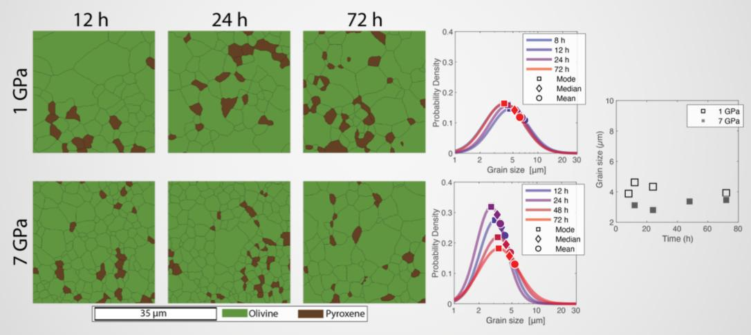
Grain growth is slower at higher pressures: Grain size distribution at 1 GPa and 12h is similar to the one at 7GPa and 72 h.
