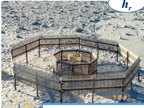
DFIR is the reference for snow measurements
