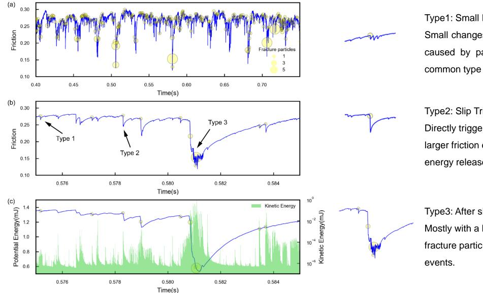
Type1: Small Disturbance Small changes in friction and energy caused by particle breakage. Most common type after breakage.
