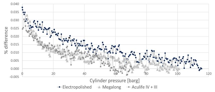
A 0.035 percent increase in amount fraction was observed with reducing pressure to zero bar and 0.015 percent on reducing the pressure to 20 bar cylinder for treated cylinders.
