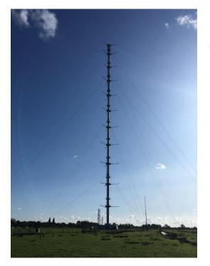
6 heights + surface TEMPERATURE WIND SPEED MOISTURE (SH, RH) HEAT FLUXES (SHF, LHF)
