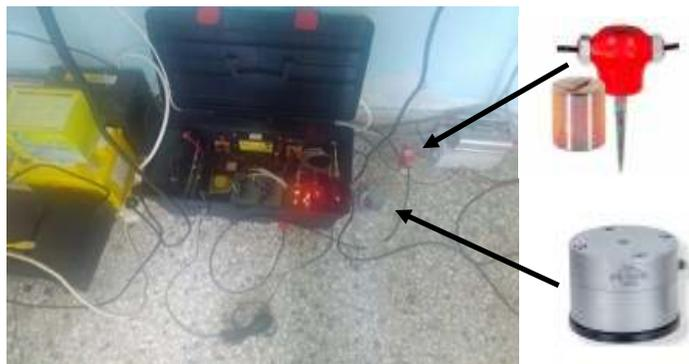
Figure 3. View of the installed low cost seismometer (black case) along with the broad band seismometer in the area of Evgiros (Lefkada island). In addition are shown: a) Velocity sensor used (Geophone GS11D – 4.5 Hz) and b) acceleration sensor used (Accelerometer KB12VD).
