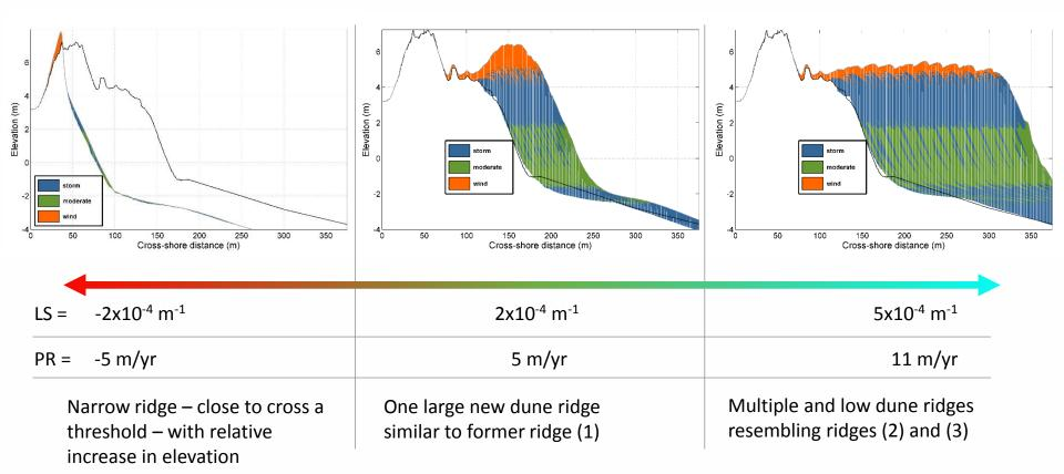
\*The calibration of modelling parameters was done using the evolution of the profile observed between 2009 and 2011. Simulations used the same parameters and the schematized meteocean conditions between 2009 and 2011 repeated 10 times to simulate 20 years of change
