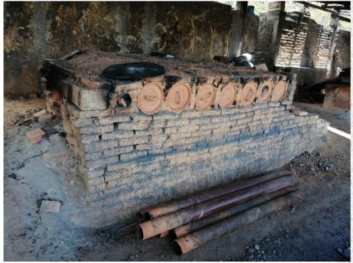
Most of this mercury mines have a rustic beneficiation plant, consisting of a furnace, where the ore is placed in decline to be burned, inside a 12-inch steel tube closed on both sides with a connection to a 4-inch tube, through which the liquid mercury and associated vapors flow to the condenser, located on one side. Once the liquid mercury is obtained, it is stored in steel containers.
