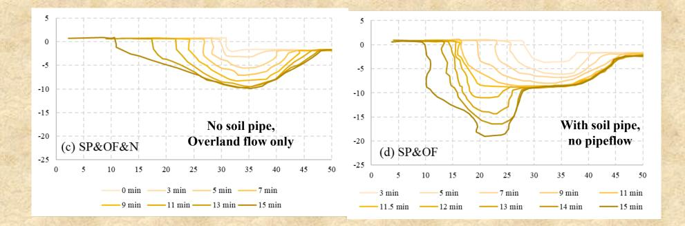
The presence of a soil pipe, even without pipe inflow, greatly changes the headcut plunge pool morphology and headcut advance.
