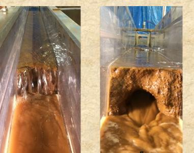
Upslope pipe inflow combined with perched water table seepage greatly shifts the outflow to pipeflow dominated
