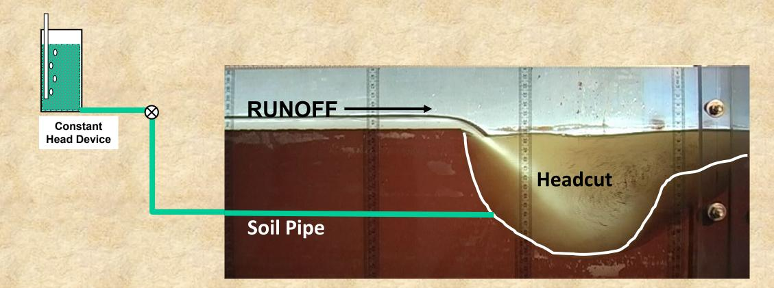
Xu et al. (2020, ESPL) modified the classic Bennett (1999, Geomorph.) headcut advance flume setup for investigation the role of pipeflow with and without surface flow
