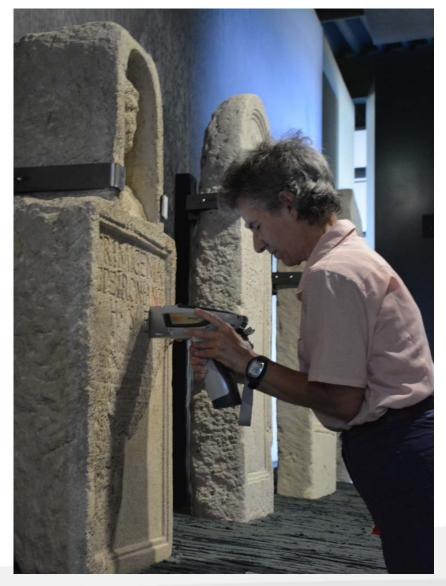
Application of XRF Analyser from AnalytiCON Instruments NITON XL3t 900s; Mining Mode Cu/Zn including light elements. Measurement period 2014-2019. Only closed dataset due to dependency on instrumentcalibration, i.e. measurements comparable only within the dataset. Interpreted data: about 630 measures of 300 archaeological stone objects and 290 measures of 155 quarry samples.
