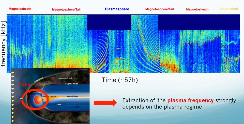
**Main goal**: Automatic detection of the electron density by the extraction of the plasma frequency ( $n_e \alpha f_{pe}^2$ )
