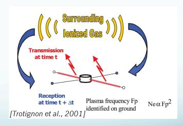
Measurement of key plasma parameters: Electron density, magnetic field amplitude
