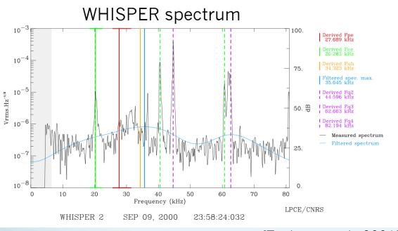
Electron plasma frequency:  $f_{pe}$  [kHz] = 9 sqrt( $n_e$  [cm<sup>-3</sup>])
