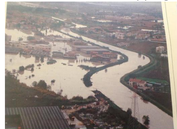
Poggio a Caiano 1992 Flood for levee overtopping
