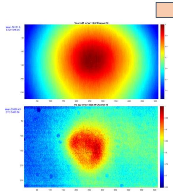
Uniformity and stray light correction for the 10<sup>th</sup> channel of the VIS camera at different aperture, focus and exposure time settings.
