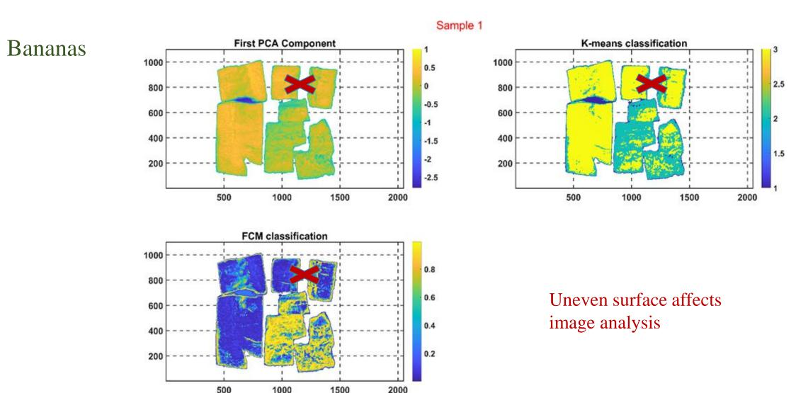
HS imaging of dried bananas samples, ripe and unripe ones. PCA, K-means and FCM were used to classify the findings.
