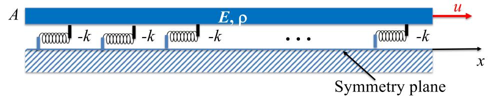
u – displacement of the rock at the fault relative to the symmetry plane (-k) – the negative spring stiffness, Pa/m
