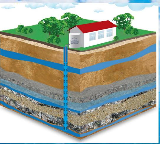
Practically, a local well drilling operator knows the geology of his region and, based on drilling mud properties and effort that the drill bit need to drill at particular depth, he is able to discriminate the cross-section and find a proper place to set the filter.
