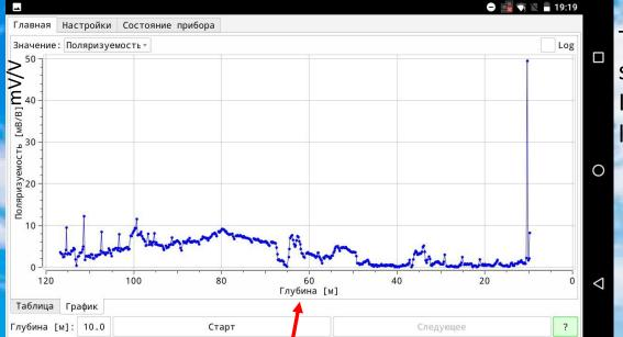
The interactive logging software screen shots are presented. IP curve is on the left, resistivity log is below.
