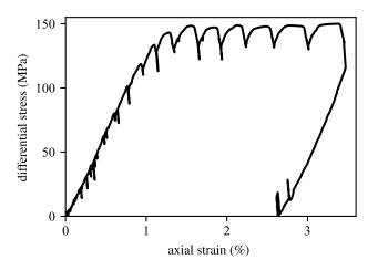
Typical of compactant cataclistic flow in porous sandstones. Large stress drops are due to relaxation during permeability measurements.
