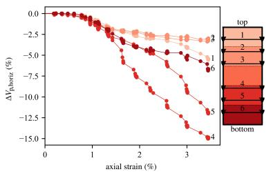
Average horizontal P wave speed across different paths. Large, early drops observed at positions 4 and 5, where permeability drop was largest.
