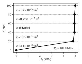
Initial permeability very heterogeneous: low permeability layer at the bottom.
