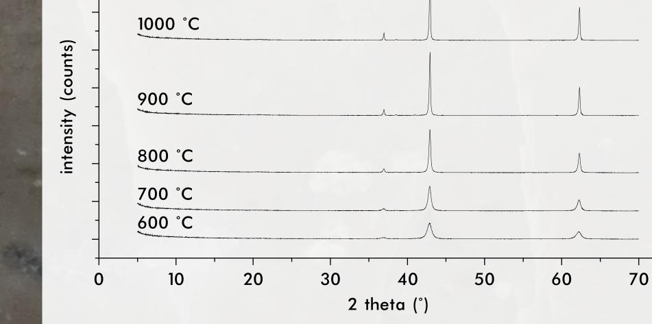
Figure 2: X-ray diffraction patterns of periclase (MgO) obtained through calcination of haydromagnesite at 600, 700, 800, 900 and 1000 °C showing an increase in peak heights and a decrease in peak widths with increasing calcination temperature.
