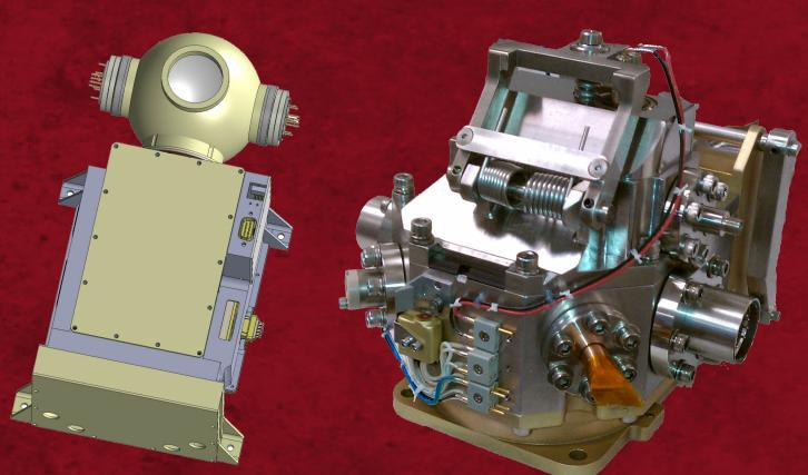
Neutral Mass Spectrometer and Ionization Gauges monitor the density and composition of Earth's thermosphere during the flight of Endurance, so that the scattering of photoelectrons can be calibrated
