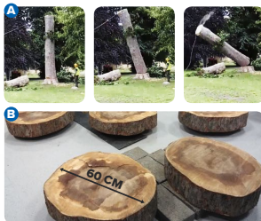
Figure 5: A) The investigated tree was brought down and subsequently B) Divided into slices for validation purposes. It is apparent that there is a dominant decay that extends along the main axis of the trunk.
