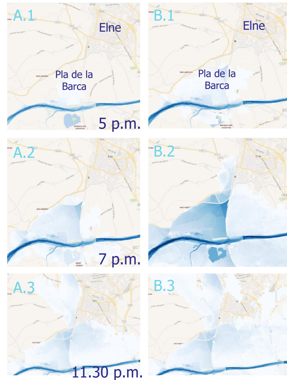
Figure 11: Comparison of the water level for the two simulations
