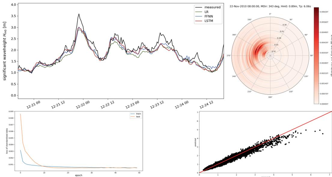
Figure 2: Top left: Reconstruction of significant wave height (model IV) for some test data. The LSTM, FFNN and LinReg are compared to the original measured data. Top right: Example of an energy density spectrum at position VST. Bottom left: Loss of the train and test data of model IV while the training process. Bottom right: Measured versus predicted significant wave height of LSTM in model IV.
