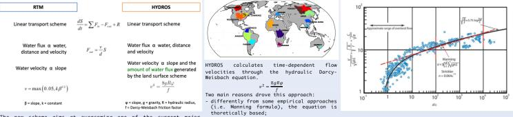
The new scheme aims at overcoming one of the current major limitations of global river routing models, that is the use of time-independent flow velocities parameterized as a function of topography. Through the imposition of hydraulic equations, HYDROS defines a time-varying flow velocity associated with the amount of lateral runoff generated by the ESM's land component and the flow through the river system.
