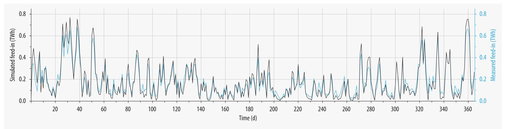
Simulated power generation and measured feed-in data [4] for the whole of Germany for 2016, aggregated from an hourly into a daily resolution.
