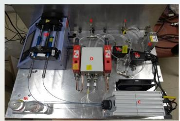
Picture of the upper stage of the instrument with the main fluidic parts
