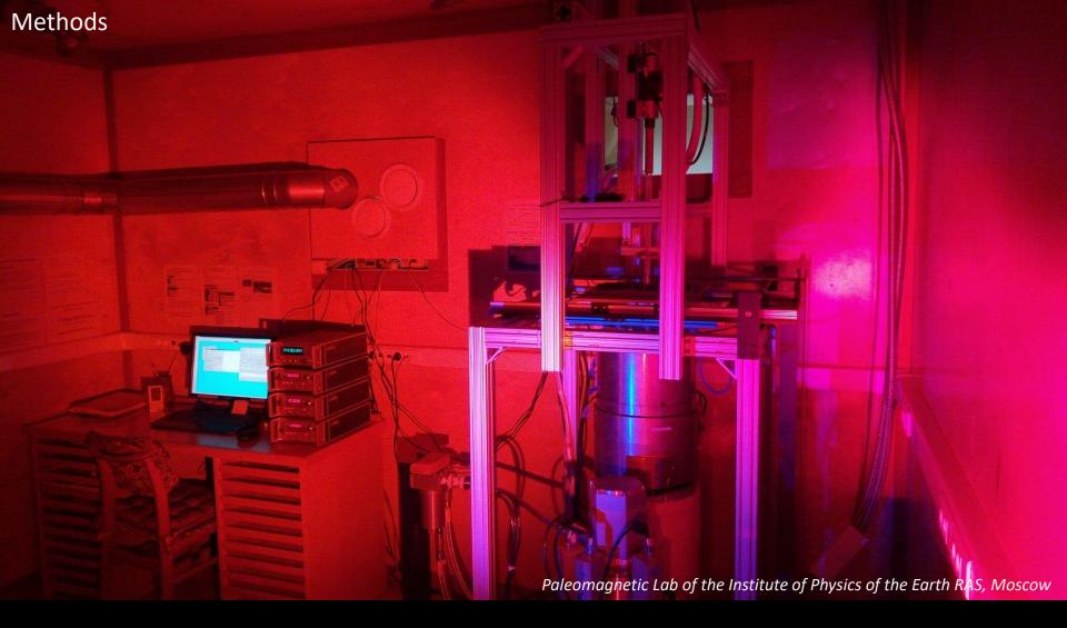
**Paleomagnetism:** 8-60 (15 in average) samples were taken from each dyke and its host rock; each sample is cut on 2 sisterspecimens (for thermal and AF demagnetization); SQUID SRM with built-in AF-demagnetizer and MMTD-80, installed in shielded room, are used; PCA analysis is the only method for getting NRM component.
