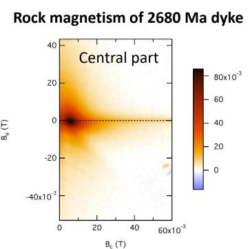
FORC diagram and thermal dependence of magnetic susceptibility curves for the 2680 Ma dyke rocks. There is no obvious difference between magnetic properties of rocks from central and marginal parts of the dyke. All rocks contain magnetite as the main carrier of ChRM.
