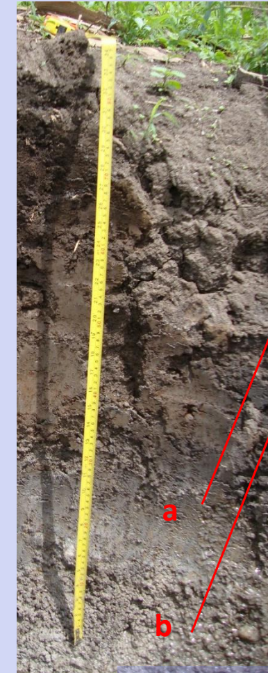
Fig. 2: Soil profile at the fringe of the wetland where interflow from the slopes can be found in a sandy loam layer (a) and in macropores of the upper part of the saprolith (b), (c) showing the horizontally layered muscovit.
