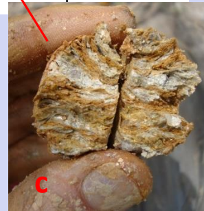
Fig. 2: Soil profile at the fringe of the wetland where interflow from the slopes can be found in a sandy loam layer (a) and in macropores of the upper part of the saprolith (b), (c) showing the horizontally layered muscovit.
