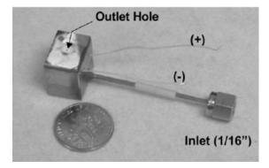
Developed at JPL 12 years ago for high-pressure gas micro-propulsion applications
