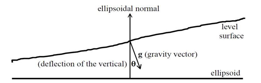
Vertical deflection represents inclination of geoid surface to reference ellipsoid surface.
