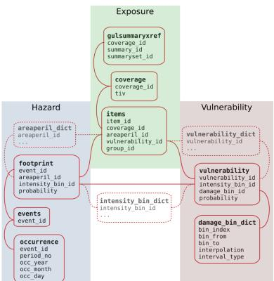
The OASIS Loss Modelling Framework (LMF) is an open source platform for developing, deploying and executing catastrophe models to enable the "plug and play" of hazard and vulnerability modules (https://oasislmf.org/).
