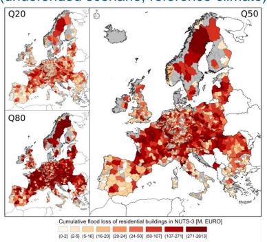
The map on the left shows the 20% quantile (Q20), the median (Q50) and the 80% quantile (Q80) of a flood loss estimation performed with BN-FLEMOps for a continent-wide 100-year flood scenario. Results are aggregated on the NUTS-3 level.
