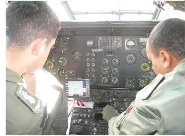
Pilot navigation panel on AS332
