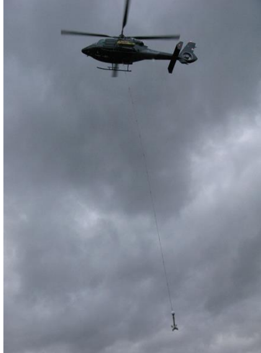
Airborne magnetic field mapping using a 'bird' deployed from an AS365 helicopter as part of an OSI test event in Hungary
