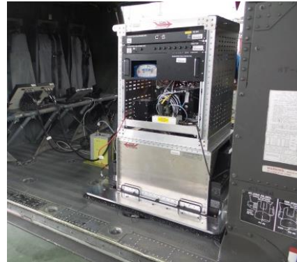
Detectors and computing on UH-60
