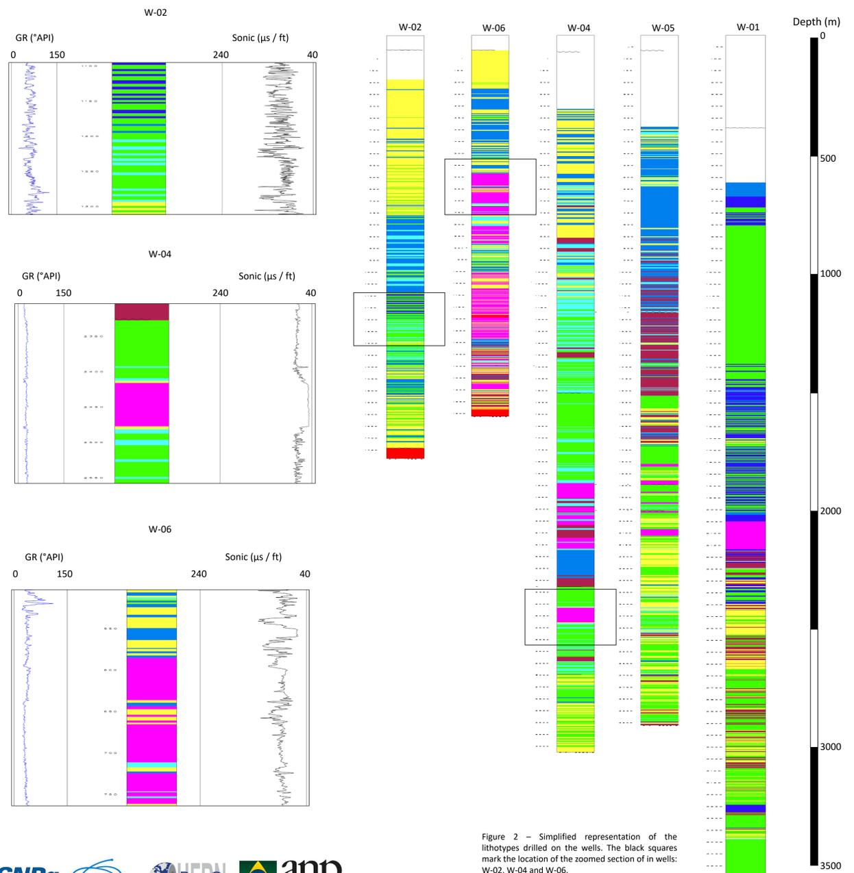
Figure 2 – Simplified representation of the lithotypes drilled on the wells. The black squares mark the location of the zoomed section of in wells: W-02, W-04 and W-06.
