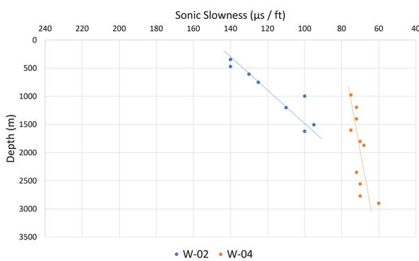
Figure 3 – Graph showing the sonic slowness curve, measured on shales, of the wells W-02 and W-04.
