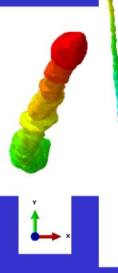
Natural period  $T_1 = 0.333$  s natural frequency  $f_1 = 3.00$  Hz Natural period  $T_2=0.312$  s natural frequency  $f_2=3.21$  Hz
